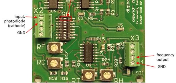
The input and output connections for this function are shown in the figure below. The anode of the photodiode must
